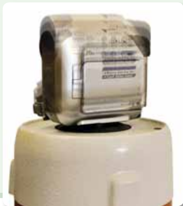
V406 shaker being used to test camcorder to ensure product reliability during operation.
